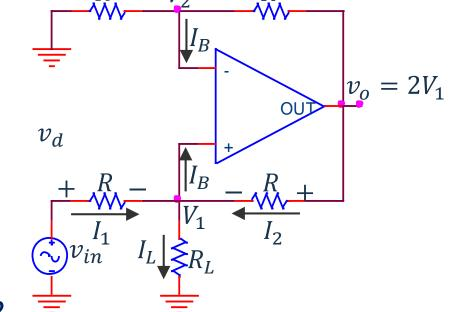
Voltage gain of the non-inverting amplifier is  $1 + \frac{R}{R} = 2$
