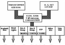
Figure 1. Layout of Power Distribution Control Room
