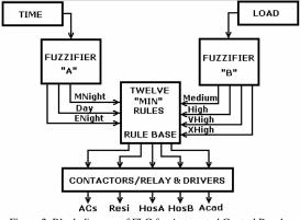
Figure 2. Block diagram of FLC for Automated Control Panel
