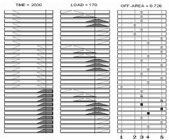
Case 4 : If TIME is ENight and LOAD is VHigh Figure 9(d). Fired rules for sample cases 4
