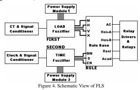
Schematic diagram of FLC is shown in the Fig. 4 consisting of two Fuzzifier modules, one rule base and two reference power supply modules.
