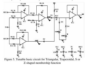
tive Slope) transfer curve and the last Op-Amp of the IC LM124 is nothing but a buffer. The input is common between both the parts while REF1 & REF2 refer to voltages specifying the start of slopes. In between, an AND gate combines both the parts and Double Clipper circuit is designed for the better shape of the curves. Resistors R3 & R4 are ganged together, while R12 & R13 are ganged together and used to tune the slopes of S and Z curves.
