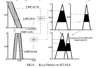
(e) Each of aggregated LMF and UMF is then computed for the Centroid as *steer\_l* and *steer\_h* using following relations:
