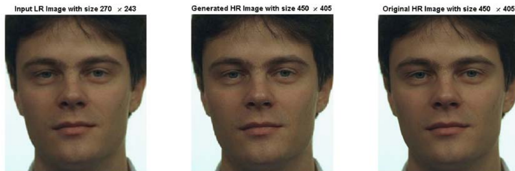
Figure 10: Result Homogeneity Technique on Color Image for resolution enhancement factor 1.667
