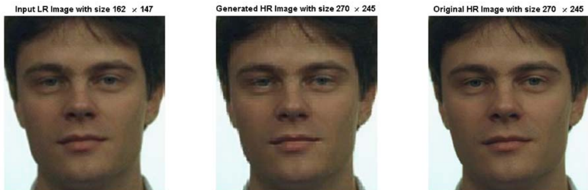
Figure 8: Result Homogeneity Technique on Color Image for resolution enhancement factor 1.667 \times 1.667 , First Stage
